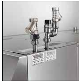
All water connections are on top and the machine has a smooth back. Since all service can be done from the front, the machine can be positioned right up against a wall, which frees up vital space in the dishwashing room.
